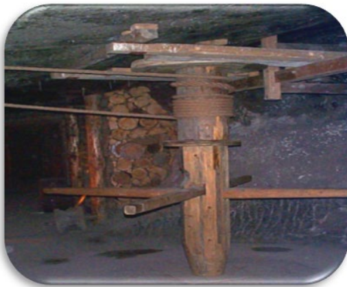
Figure 4. Winch System, Cracow Saltworks Museum Source: Wikipedia, 2025
